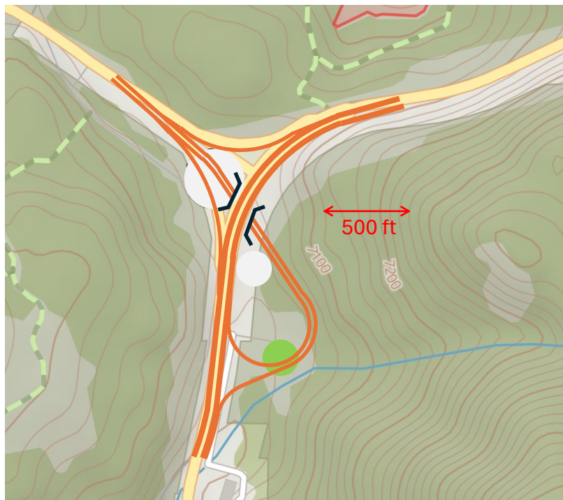
Figure 3. Suggested Trumpet Interchange Design at US 50 and SR20 Intersection near Spoooner Summit (OpenStreetMap 3 )
